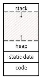
The address space is represented graphically on the left. The lowest address is at the bottom and the highest address is at the top. It contains the following four regions:
