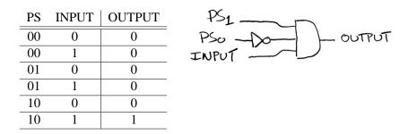
In this case, the circuit should output a 1 if and only if the input pattern is 101. The circuit for that purpose essentially just matches the 101 pattern, when a match occurs, it outputs a 1—for all other input patterns it outputs a 0. Try it!
