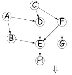
[A,B,C,F,D,G,E,H], or [A,C,B,D,F,E,G,H], or [A,B,C,F,D,E,H,G], or : Set<Vertex> fringe; fringe = set of all nodes with no predecessors; while (! fringe.isEmpty()) { Vertex v = fringe.removeOne (); add v to end of result list; For each edge (v,w) { decrease predecessor count of w; if (predecessor count of w == 0) fringe.add (w); } }
