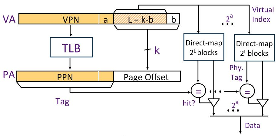
After the PPN is known, 2<sup>a</sup> physical tags are compared How does this scheme scale to larger caches?
