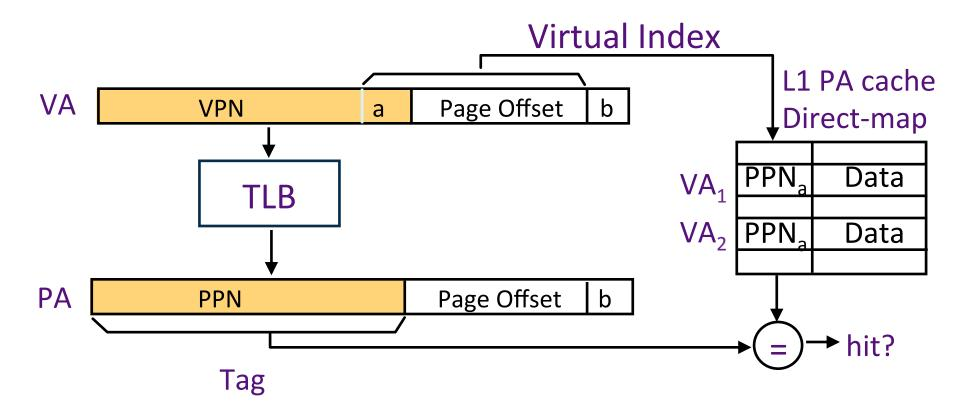
Can VA<sub>1</sub> and VA<sub>2</sub> both map to PA?
