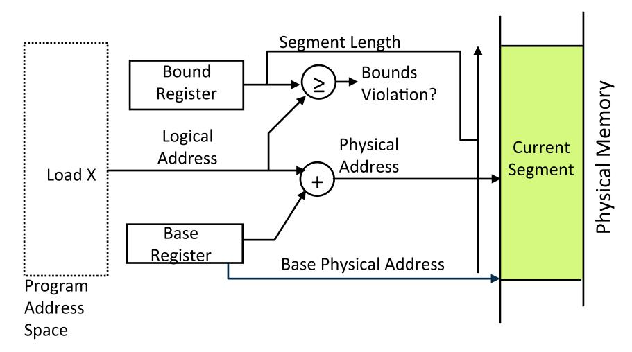
Base and bounds registers are visible/accessible only when processor is running in the *supervisor mode*
