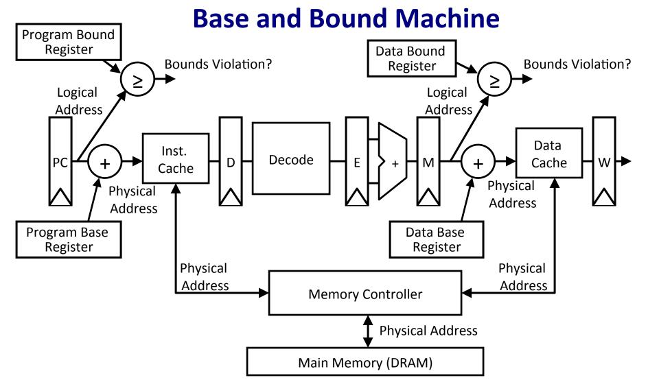
Can fold addition of base register into (register+immediate) address calculation using a carry-save adder (sums three numbers with only a few gate delays more than adding two numbers)
