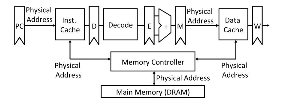
In a bare machine, the only kind of address is a physical address, corresponding to address lines of actual hardware memory.
