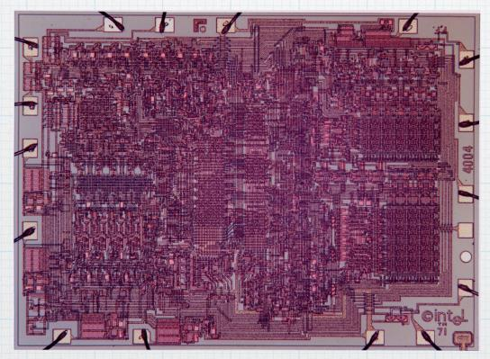
The Intel 4004 microprocessor, which was introduced in 1971. The 4004 contained 2300 transistors and performed 60,000 calculations per second. Courtesy: Intel.
