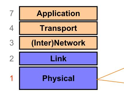
Encoding bits to send them over a <u>single</u> **physical link** e.g. patterns of *voltage levels / photon intensities / RF modulation*
