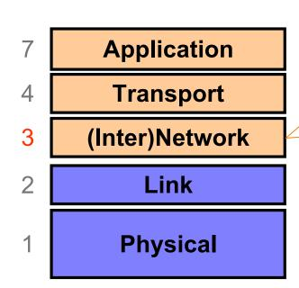
Bridges multiple "subnets" to provide *end-to-end* internet connectivity between nodes • Provides <u>global</u> addressing
