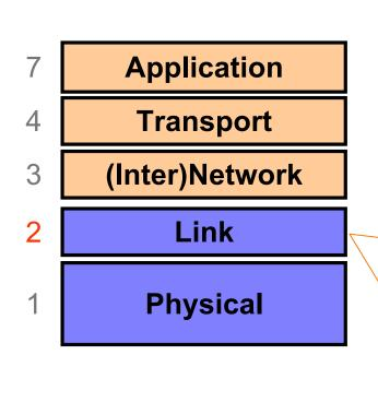
Framing and transmission of a collection of bits into individual messages sent across a single "subnetwork" (one physical technology)
