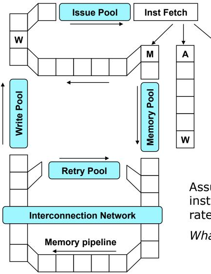
• Every cycle, one VLIW instruction from one active thread is launched into pipeline
