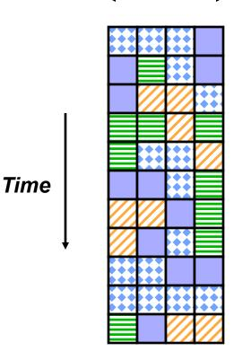
Interleave multiple threads to multiple issue slots with no restrictions
