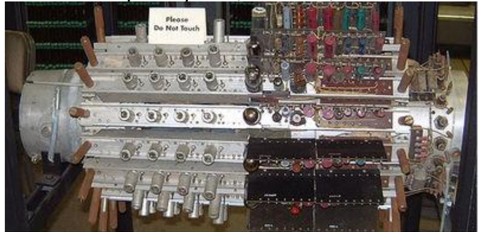
Mercury Delay Line, Univac 1, 1951
