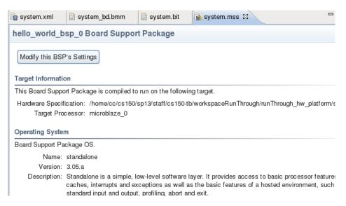
Click the *Modify this BSP's Settings* button and you can see an overview of the OS and the hardware platform we use. In this lab, to keep things simple, we only have a basic software layer (standalone) instead of a fully functional OS. Click *standalone* under *Overview* to bring up the screen below.
