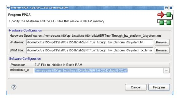
To program the FPGA, use the bitstream and BMM file from the exported hardware platform. For the software configuration, choose <code>GCD.elf</code> in the GCD project under <code>GCD/Debug</code>. Click *Program* to configure the FPGA and load the gcd program.
