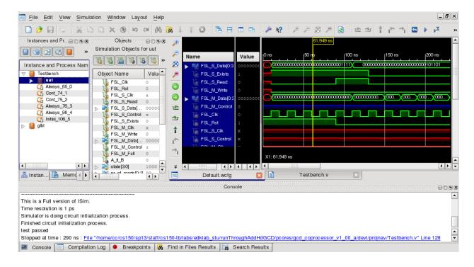
After verifying the functionality of your module, go back to XPS. As the hardware platform has been changed, select *Hardware → Clean Bitstream*, and press *Export Design* in the *Navigator*. Choose *Export & Launch SDK*. After the hardware compilation, when SDK is launched again, the BSPs in the original workspace will be automatically updated. Then the coprocessor is ready for use by your software application.
