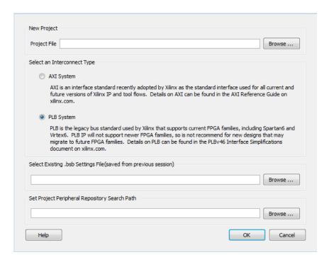
Click the *Browse* button under *New Project* and specify a location for the new project file (system.xmp). Make sure the PLB system is selected under *Interconnect Type*. To facilitate the creation of systems on our FPGA board, a board definition file is provided in the lab distribution. To point the tool to this file, under *Set Project Peripheral Repository Search Path*, choose the lib directory in the lab distribution (lab5B/). Press OK to create the new project.
