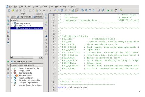
In the *Hierarchy* view of the project (on the left of the screen), double click the gcd\_coprocessor module to open up the Verilog file in the HDL editor of ISE.
