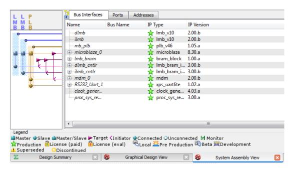
From the System Assembly View, you can see a MicroBlaze based system with the specified peripherals has been generated, and all the connections between components are created accordingly. The local memory bus (LMB) is used by the MicroBlaze core to control the dlmb\_cntlr and ilmb\_cntlr modules (the microblaze\_0 is the master while the controlled modules are the slaves). Meanwhile, the PLB bus is used to connect to the RS232\_Uart\_1 component.
