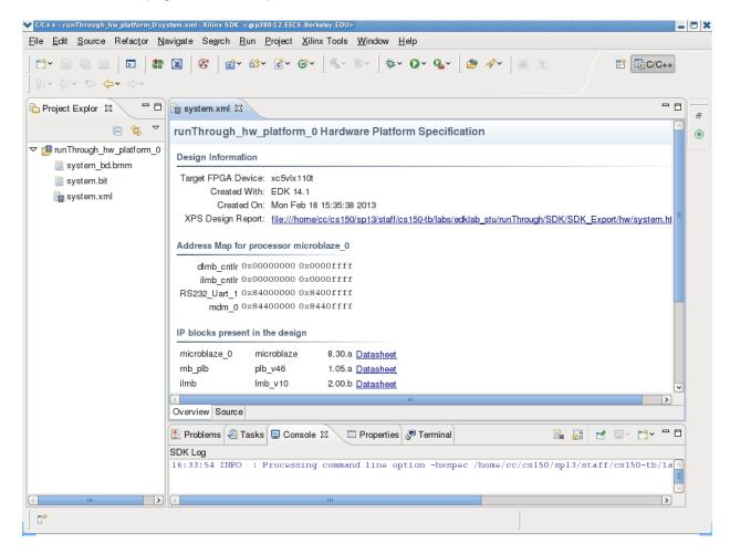
There are three files used to capture the information of the exported hardware platform. The system.xml file contains the information about the IP cores used in the design. The system.bit file is used for programming the FPGA device while the system\_bd.bmm file is used by the SDK for loading memory onto the target board. When we create a software project in Xilinx SDK, we will need to refer to the hardware platform the compiled program is meant to run on.
