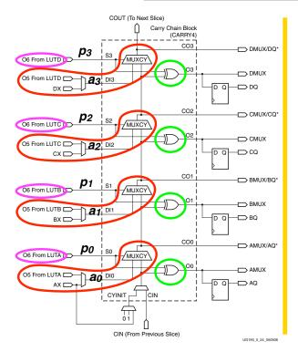
We can map ripple-carry addition onto carry-chain block.
