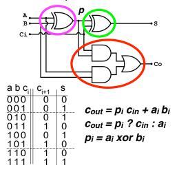
The carry-chain block also useful for speeding up other adder structures and counters.
