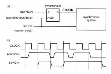
• The D flip-flop samples the asynchronous input at each cycle and produces a synchronous output that meets the setup time of the next stage.
