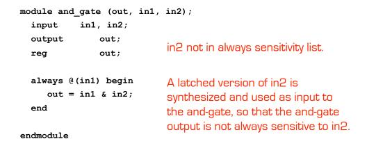
Easy way to avoid incomplete triggers for combinational logic is with: always @\*
