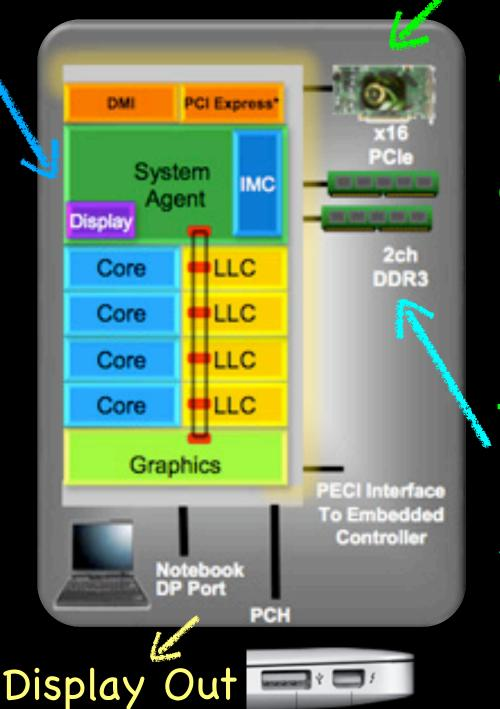
**PCIe** bus supports discrete GPU, with dedicated RAM and monitor outputs. IGP uses system DRAM as graphics memory.
