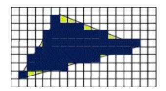
Then, create "pixel fragments" to fill in the triangle (rasterization).
