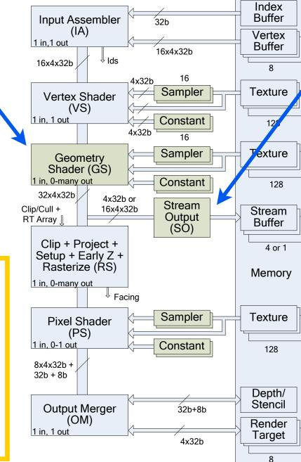
Stream Output: Lets vertex stream recirculate through shaders many times ... (and also, back to CPU)
