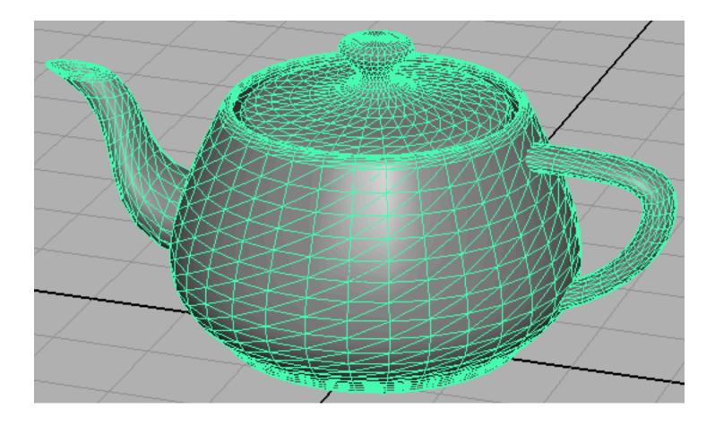
A teapot (famous object in computer graphics history). A "wire-frame" of triangles can capture the 3-D shape of complex, man-made objects.
