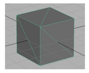
A cube whose faces are made up of triangles. This is a 3-D model of a cube -- model includes faces we can't see in this view.
