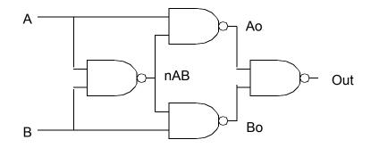
Write the same behavior as a behavioral module using continuous assignment.
