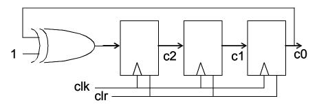
Generate the truth table how this counter "increments". This has four input columns (clr, c2, c1, and c0) and three output columns (the new c2, c1, and c0).
