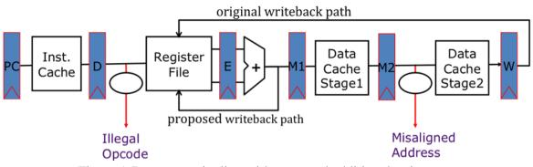
Figure 1-B. 6-stage pipeline with proposed additional write port.
