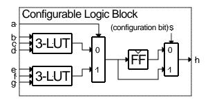
The easiest way to use the CLB is as a 4-LUT. We compose the 4-LUT from the pair of 3-LUTs by feeding the same 3 inputs into  $\{b,c,d\}$  as into  $\{e,f,g\}$  and by using *a* for the fourth input. The first 3-LUT implements the 4-LUT function assuming *a*=0 while the second assumes *a*=1. This technique is demonstrated in Homework #3, problem 3.
