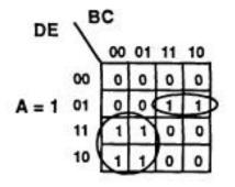
$f(A, B, C, D, E) = A \overline{B} D + \overline{A} \overline{B} \overline{D} \overline{E} + A B \overline{D} E$ Eleven literals
