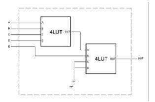
This takes 5 inputs, has one output, and is made completely from programmable 4-LUTs. But it is not a complete 5-LUT; it cannot perform any function of 5 inputs.
