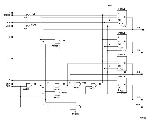
Figure 11-17 X74\_160 Implementation XC4000E, XC4000X, XC5200, Spartan, SpartanXL
