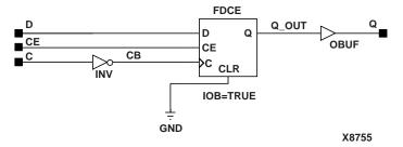
Figure 8-43 OFDX 1 Implementation Spartan2, Virtex
