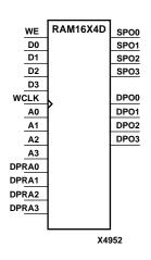
RAM16X4D is a 16-word by 4-bit static dual port random access memory with synchronous write capability. The device has two separate address ports: the read address (DPRA3 – DPRA0) and the write address (A3 – A0). These two address ports are completely asynchronous. The read address controls the location of data driven out of the output pin (DPO3 – DPO0), and the write address controls the destination of a valid write transaction.
