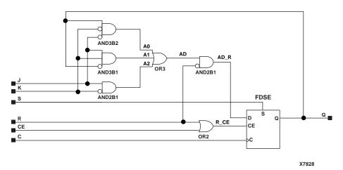
Figure 5-46 FJKSRE Implementation XC3000, XC4000E, XC4000X, XC5200, Spartan, SpartanXL, Spartan2, Virtex
