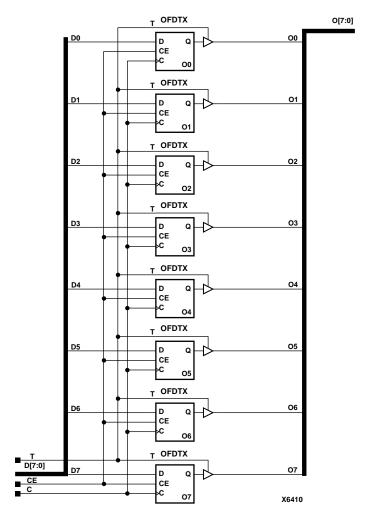
Figure 8-37 OFDTX8 Implementation XC4000E, XC4000X, Spartan, SpartanXL
