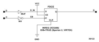
Figure 6-9 IFD\_1 Implementation XC5200, Spartan2, Virtex
