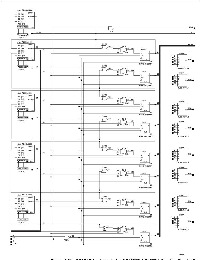
Figure 4-21 CC8CLE Implementation XC4000E, XC4000X, Spartan, SpartanXL
