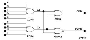
Figure 11-34 X74\_280 Implementation XC3000, XC4000E, XC4000X, XC5200, Spartan, SpartanXL
