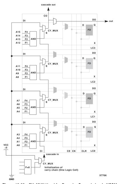
Figure 12-22 CY\_MUX Used for Decoder Cascade Logic XC5200
