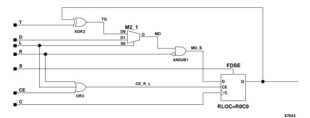
Figure 5-71 FTSRLE Implementation XC3000, XC4000E, XC4000X, XC5200, Spartan, SpartanXL, Spartan2, Virtex
