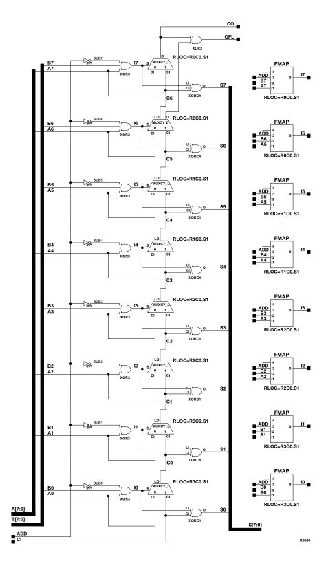
Figure 3-20 ADSU8 Implementation Spartan2, Virtex
