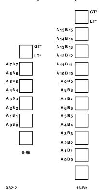
In the process of combining the logic that loads GT and LT, the place and route software might map the logic that generates GT and LT to different function generators. If this mapping occurs, the GT and LT logic cannot be placed in the uppermost CLB, as indicated in the illustration.
