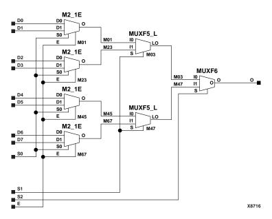
Figure 7-23 M8\_1E Implementation Spartan2, Virtex
