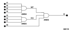
Figure 3-26 AND8 Implementation XC4000E, XC4000X, Spartan, SpartanXL
