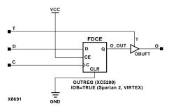
Figure 8-30 OFDT Implementation XC5200, Spartan2, Virtex
