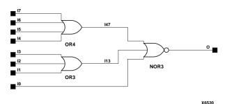
Figure 7-38 NOR8 Implementation XC4000E, XC4000X, Spartan, SpartanXL
