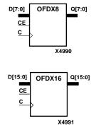
OFDX, OFDX4, OFDX8, and OFDX16 are single and multiple output D flip-flops. The flip-flops are located in an input/output block (IOB) for XC4000E. The Q outputs are connected to OPADs or IOPADs. The data on the D inputs is loaded into the flip-flops during the Low-to-High clock (C) transition and appears on the Q outputs. When CE is Low, flip-flop outputs do not change.
