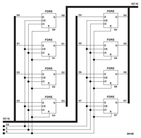
Figure 5-9 FD8RE Implementation XC3000, XC4000E, XC4000X, XC5200, XC9000, Spartan, SpartanXL, Spartan2, Virtex
