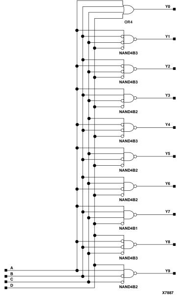
Figure 11-1 X74\_42 Implementation XC3000, XC4000E, XC4000X, XC5200, XC9000, Spartan, SpartanXL
