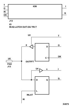
Figure 6-47 XC3000 IOB Primitive Example and Equivalent Circuit
