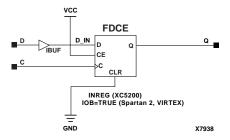
Figure 6-5 IFD Implementation XC5200, Spartan2, Virtex
