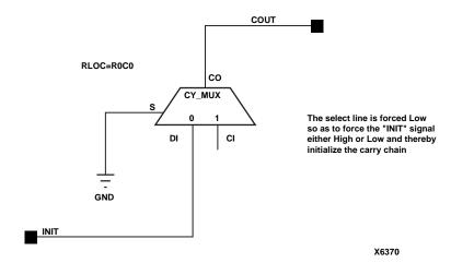
Figure 4-52 CY INIT 4-Bit Adder Implementation XC5200
