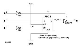
Figure 8-17 OFDE\_1 Implementation XC5200, Spartan2, Virtex
