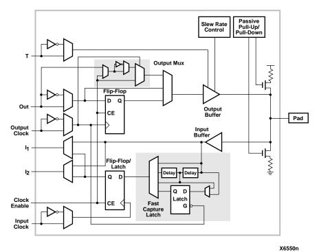
Figure 6-44 Block Diagram of XC4000X IOB
