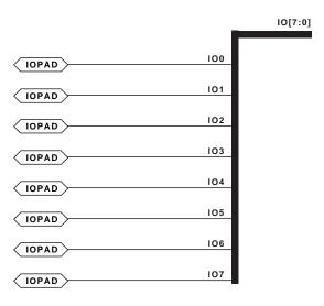
Figure 6-48 IOPAD8 Implementation XC3000, XC4000E, XC4000X, XC5200, XC9000, Spartan, SpartanXL, Spartan2, Virtex
