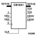
CB2X1, CB4X1, CB8X1, and CB16X1 are, respectively, 2-, 4-, 8-, and 16-bit (stage), synchronously loadable, asynchronously clearable, bidirectional binary counters. These counters have separate count-enable inputs and synchronous terminal-count outputs for up and down directions to support high-speed cascading in the CPLD architecture.
