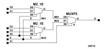
Figure 7-21 M4\_1E Implementation Spartan2, Virtex
