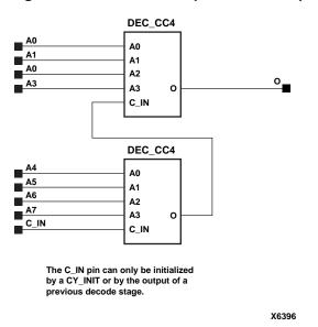
Figure 4-59 DEC\_CC8 Implementation XC5200, Spartan2, Virtex
