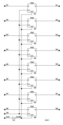
Figure 11-33 X74\_273 Implementation XC3000, XC4000E, XC4000X, XC5200, XC9000, Spartan, SpartanXL
