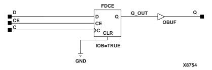
Figure 8-40 OFDX Implementation Spartan2, Virtex
