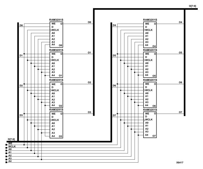
Figure 9-7 RAM32X8S Implementation XC4000E, XC4000X, Spartan, Spartan2, SpartanXL, Virtex
