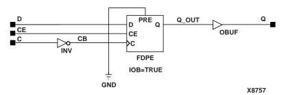
Figure 8-46 OFDXI 1 Implementation Spartan2, Virtex
