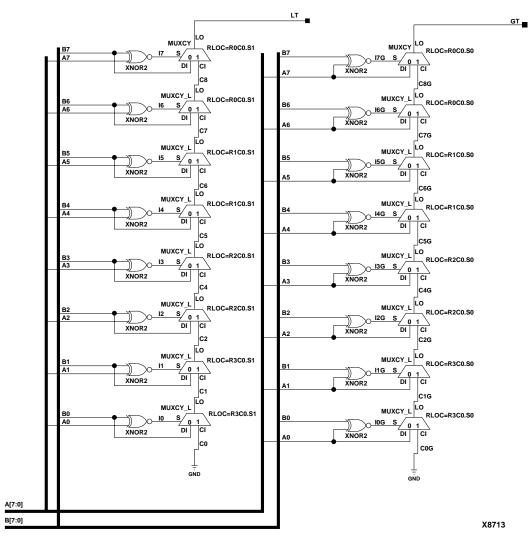
Figure 4-48 COMPMC8 Implementation Spartan2, Virtex
