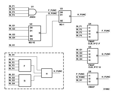
Figure 6-2 Partitioning Logic Using FMAP and HMAP Symbols
