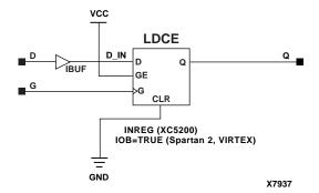
Figure 6-24 ILD Implementation XC5200, Spartan2, Virtex
