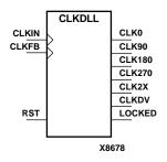
CLKDLL is a clock delay locked loop used to minimize clock skew. CLKDLL synchronizes the clock signal at the feed back clock input (CLKFB) to the clock signal at the input clock (CLKIN). The locked output (LOCKED) is high when the two signals are in phase. The signals are considered to be in phase when their rising edges are within 250 ps of each other.
