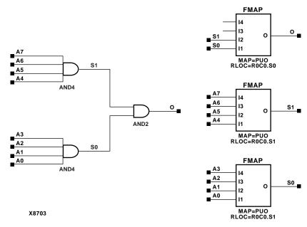
Figure 4-63 DECODE8 Implementation Spartan2, Virtex
