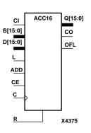
ACC4, ACC8, ACC16 can add or subtract a 4-, 8-, 16-bit unsigned-binary, respectively or twos-complement word to or from the contents of a 4-, 8-, 16-bit data register and store the results in the register. The register can be loaded with the 4-, 8-, 16-bit word.
