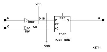
Figure 6-13 IFDI\_1 Implementation Spartan2, Virtex
