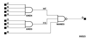
Figure 7-28 NAND8 Implementation XC4000E, XC4000X, Spartan, SpartanXL
