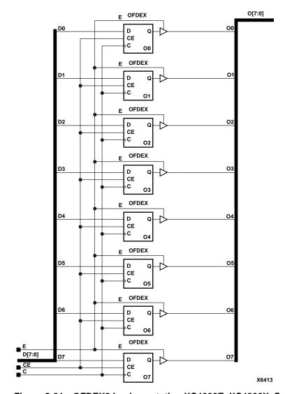
Figure 8-21 OFDEX8 Implementation XC4000E, XC4000X, Spartan, SpartanXL
