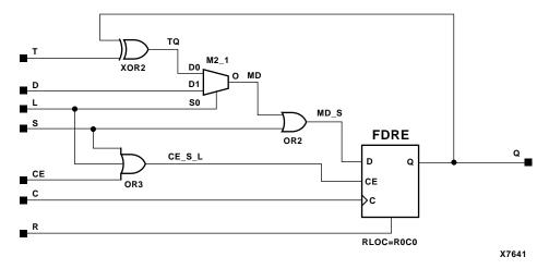
Figure 5-67 FTRSLE Implementation XC3000, XC4000E, XC4000X, XC5200, Spartan, SpartanXL, Spartan2, Virtex
