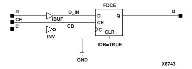
Figure 6-17 IFDX\_1 Implementation Spartan2, Virtex
