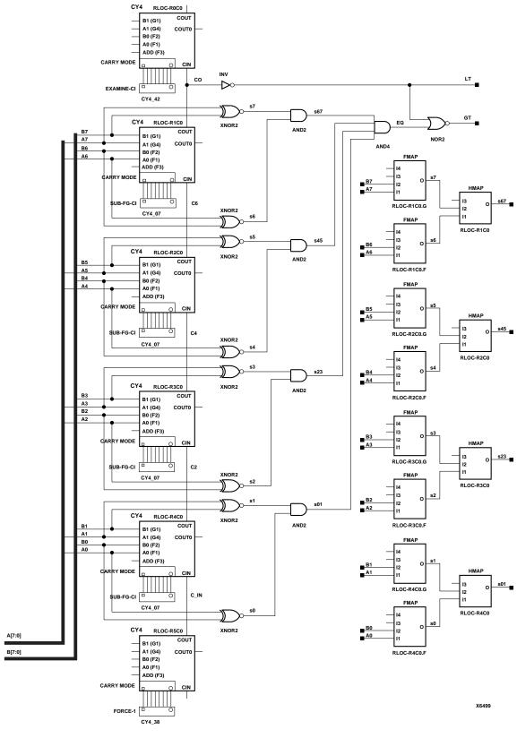
Figure 4-46 COMPMC8 Implementation XC4000E, XC4000X, Spartan, SpartanXL
