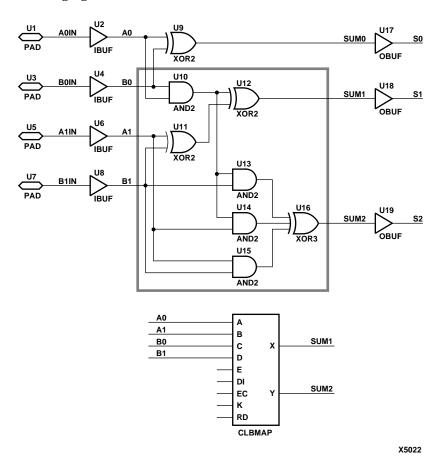
Figure 4-42 XC3000 CLBMAP Primitive Example and Equivalent
