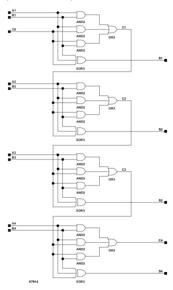
Figure 11-36 X74\_283 Implementation XC3000, XC4000E, XC4000X, XC5200, Spartan, SpartanXL
