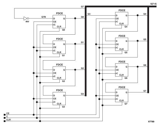
Figure 4-39 CJ8CE Implementation XC3000, XC4000E, XC4000X, XC5200, XC9000, Spartan, SpartanXL, Spartan2, Virtex
