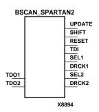
The BSCAN\_SPARTAN2 symbol is used to create internal boundary scan chains in a Spartan2 device. The 4-pin JTAG interface (TDI, TDO, TCK, and TMS) are dedicated pins in Spartan2. To use normal JTAG for boundary scan purposes, just hook up the JTAG pins to the port and go. The pins on the BSCAN\_SPARTAN2 symbol do not need to be connected, unless those special functions are needed to drive an internal scan chain.
