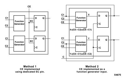
Figure 1-3 Clock Enable Implementation Methods
