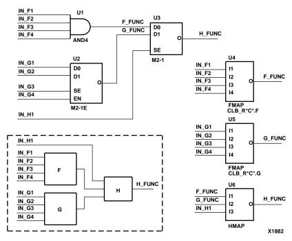
Figure 5-48 Partitioning Logic Using FMAP and HMAP Symbols
