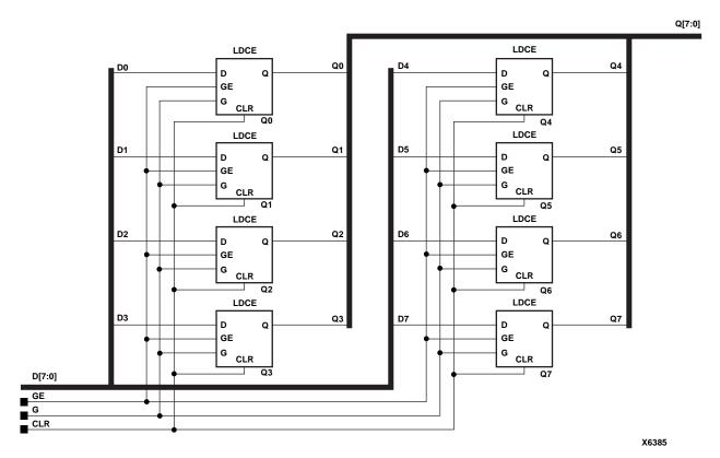
Figure 7-14 LD8CE Implementation XC4000X, XC5200, SpartanXL, Spartan2, Virtex
