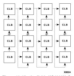
Figure 12-17 Available XC4000X, Spartan, and SpartanXL Carry Propagation Paths (dotted lines use general interconnect)
