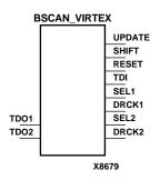
The BSCAN\_VIRTEX symbol is used to create internal boundary scan chains in a Virtex device. The 4-pin JTAG interface (TDI, TDO, TCK, and TMS) are dedicated pins in Virtex. To use normal JTAG for boundary scan purposes, just hook up the JTAG pins to the port and go. The pins on the BSCAN\_VIRTEX symbol do not need to be connected, unless those special functions are needed to drive an internal scan chain.
