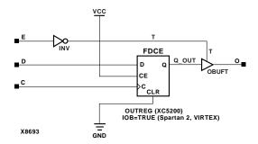
Figure 8-13 OFDE Implementation XC5200, Spartan2, Virtex
