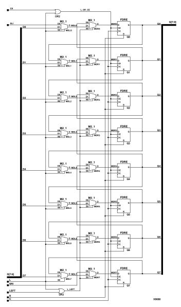
Figure 10-10 SR8RLED Implementation XC3000, XC4000E, XC4000X, XC5200, XC9000, Spartan, SpartanXL, Spartan2, Virtex
