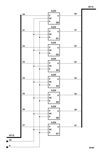
Figure 6-38 ILDX8 Implementation XC4000E, XC4000X, Spartan, SpartanXL, Spartan2, Virtex
