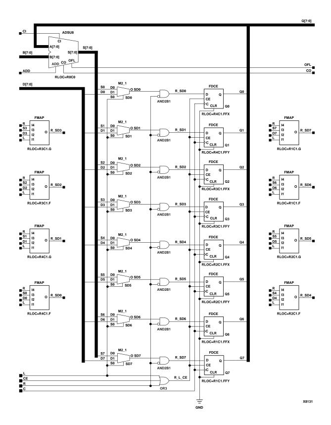
Figure 3-3 ACC8 Implementation XC4000E, XC4000X, Spartan, SpartanXL
