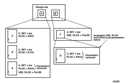
Figure 12-13 Using the USE\_RLOC Constraint to Control RLOC Application on U SET Sets
