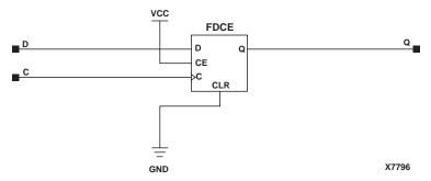
Figure 5-4 FD Implementation XC3000, XC4000E, XC4000X, XC5200, Spartan, SpartanXL
