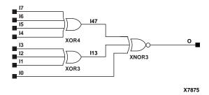
Figure 10-21 XNOR8 Implementation XC4000E, XC4000X, XC5200, Spartan, SpartanXL
