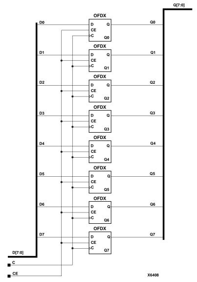
Figure 8-41 OFDX8 Implementation XC4000E, XC4000X, Spartan, SpartanXL, Spartan2, Virtex
