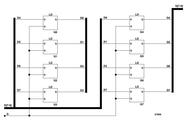
Figure 7-6 LD8 Implementation XC4000X, XC9000, SpartanXL, Spartan2, Virtex
