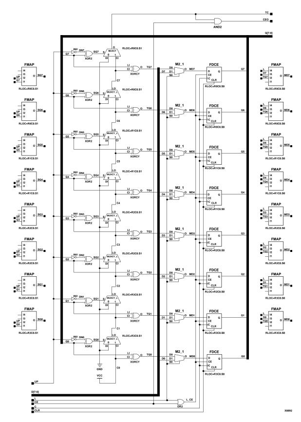
Figure 4-26 CC8CLED Implementation Spartan2, Virtex
