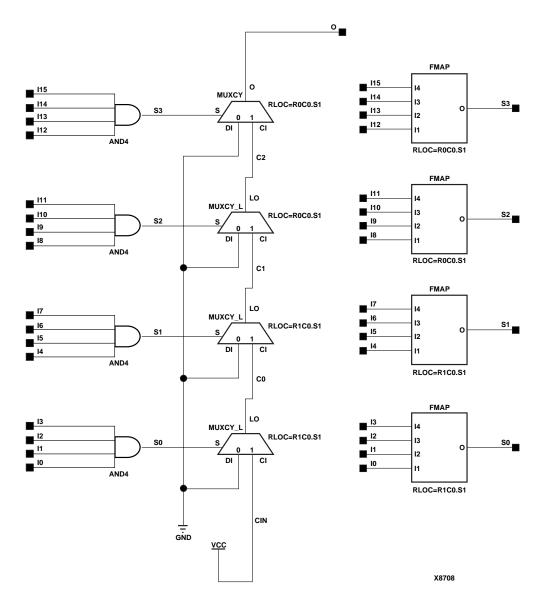
Figure 3-32 AND16 Implementation Spartan2, Virtex
