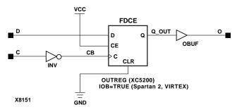
Figure 8-11 OFD\_1 Implementation XC5200, Spartan2, Virtex
