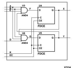
Figure 4-41 XC3000 CLB Primitive Example and Equivalent Circuit
