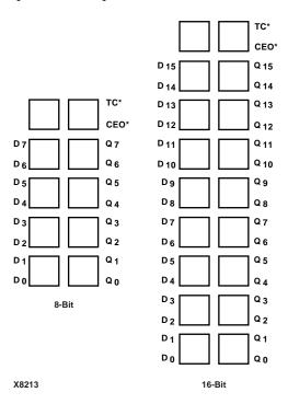
In the process of combining the logic that loads CEO and TC, the place and route software might map the logic that generates CEO and TC to different function generators. If this mapping occurs, the CEO and TC logic cannot be placed in the uppermost CLB as indicated in the illustration.
