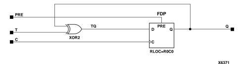
Figure 5-59 FTP Implementation XC4000E, XC4000X, XC5200, Spartan, SpartanXL, Spartan2, Virtex
