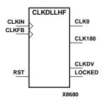
CLKDLLHF is a high frequency clock delay locked loop used to minimize clock skew. CLKDLLHF synchronizes the clock signal at the feed back clock input (CLKFB) to the clock signal at the input clock (CLKIN). The locked output (LOCKED) is high when the two signals are in phase. The signals are considered to be in phase when their rising edges are within 250 ps of each other.
