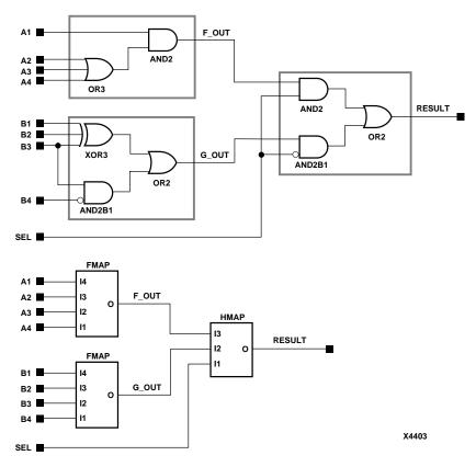
Figure 12-2 FMAP and HMAP Schematics
