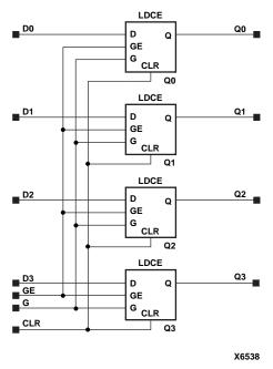
Figure 7-13 LD4CE Implementation XC4000X, XC5200, SpartanXL, Spartan2, Virtex
