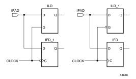
Figure 6-22 Legal Combinations of IFD and ILD for a Single IOB in XC4000E, XC4000X, Spartan, or SpartanXL
