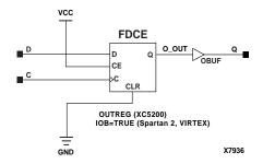
Figure 8-6 OFD Implementation XC5200, Spartan2, Virtex
