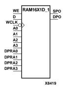
RAM16X1D\_1 is a 16-word by 1-bit static dual port random access memory with synchronous write capability and negative-edge clock. The device has two separate address ports: the read address (DPRA3 – DPRA0) and the write address (A3 – A0). These two address ports are completely asynchronous. The read address controls the location of the data driven out of the output pin (DPO), and the write address controls the destination of a valid write transaction.
