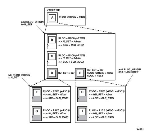
Figure 12-15 Using an RLOC\_ORIGIN to Modify H\_SET and HU\_SET Sets
