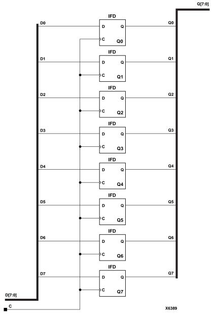
Figure 6-7 IFD8 Implementation XC3000, XC4000E, XC4000X, XC5200, XC9000, Spartan, SpartanXL, Spartan2, Virtex
