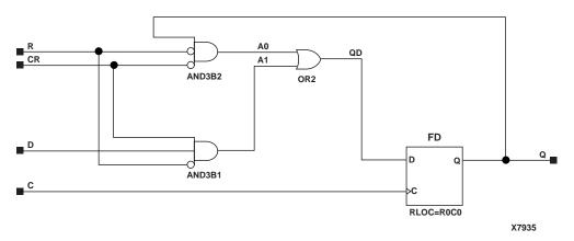
Figure 5-21 FDRE Implementation XC3000, XC4000E, XC4000X, XC5200, Spartan, SpartanXL
