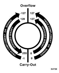
Figure 3-16 ADSU Carry-Out and Overflow Boundaries
