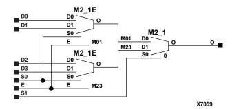
Figure 7-20 M4\_1E Implementation XC3000, XC4000E, XC4000X, XC5200, XC9000, Spartan, SpartanXL
