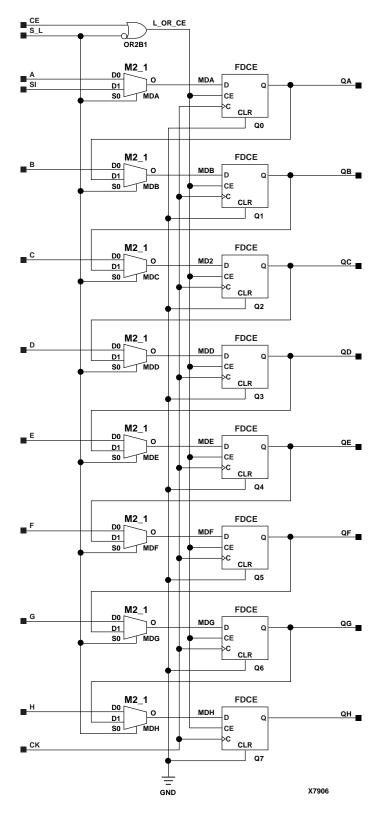
Figure 11-26 X74\_165S Implementation XC3000, XC4000E, XC4000X, XC5200, XC9000, Spartan, SpartanXL
