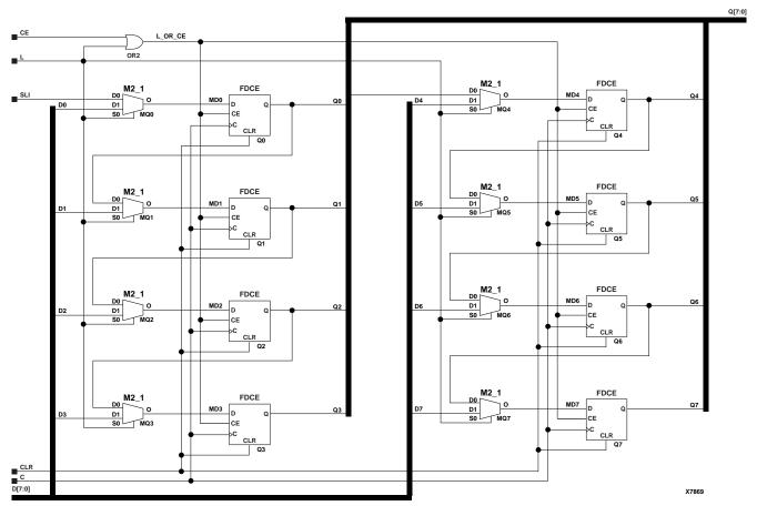
Figure 10-5 SR8CLE Implementation XC3000, XC4000E, XC4000X, XC5200, XC9000, Spartan, SpartanXL, Spartan2, Virtex
