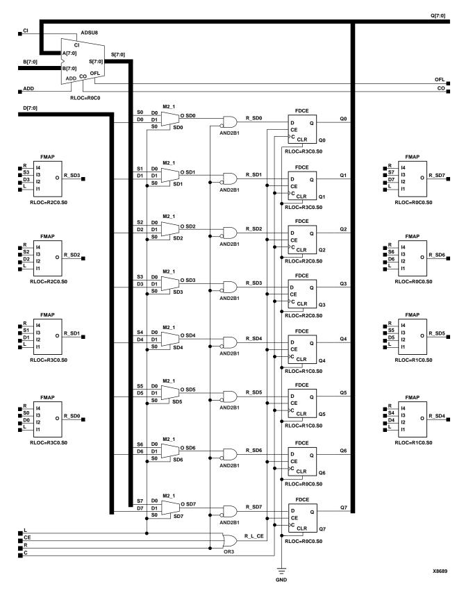
Figure 3-5 ACC8 Implementation Spartan2, Virtex
