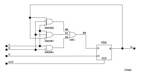
Figure 5-34 FJKC Implementation XC3000, XC4000E, XC4000X, XC5200, Spartan, SpartanXL, Spartan2, Virtex
