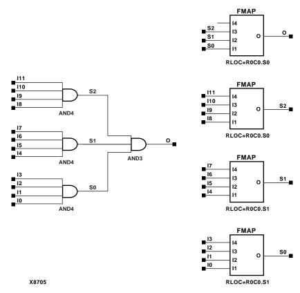
Figure 3-30 AND12 Implementation Spartan2, Virtex
