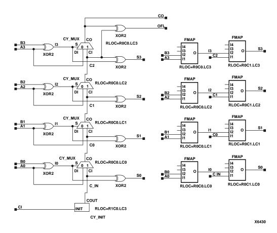
Figure 4-53 CY\_MUX 4-Bit Adder Schematic XC5200
