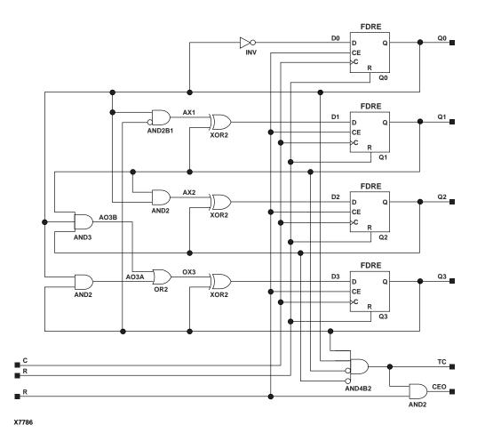
Figure 4-35 CD4RE Implementation XC3000, XC4000E, XC4000X, XC5200, Spartan, SpartanXL, Spartan2, Virtex
