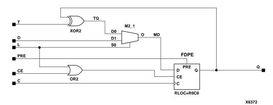
Figure 5-63 FTPLE Implementation XC4000E, XC4000X, XC5200, Spartan, SpartanXL, Spartan2, Virtex
