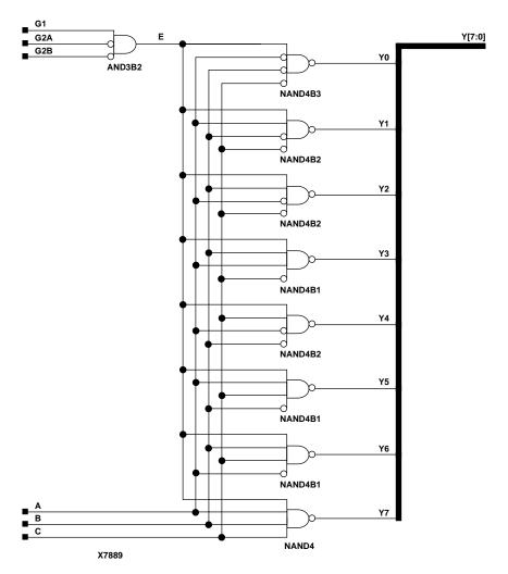
Figure 11-4 X74\_138 Implementation XC3000, XC4000E, XC4000X, XC5200, XC9000, Spartan, SpartanXL
