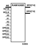
RAM16X8D is a 16-word by 8-bit static dual port random access memory with synchronous write capability. The device has two separate address ports: the read address (DPRA3 – DPRA0) and the write address (A3 – A0). These two address ports are completely asynchronous. The read address controls the location of data driven out of the output pin (DPO7 – DPO0), and the write address controls the destination of a valid write transaction.
