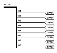
Figure 8-47 OPAD8 Implementation XC3000, XC4000E, XC4000X, XC5200, XC9000, Spartan, SpartanXL, Spartan2, Virtex
