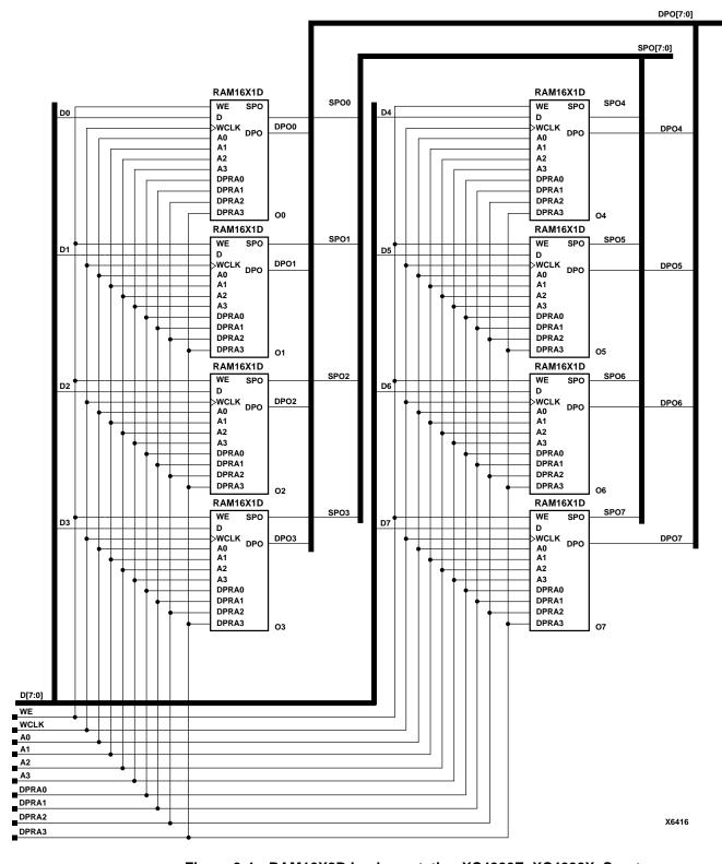
Figure 9-4 RAM16X8D Implementation XC4000E, XC4000X, Spartan, SpartanXL
