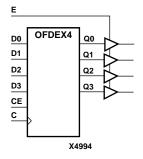
The flip-flops are asynchronously cleared with Low outputs when power is applied. FPGAs simulate power-on when global set/reset (GSR) is active. GSR defaults to active-High but can be inverted by adding an inverter in front of the GSR input of the STARTUP symbol.
