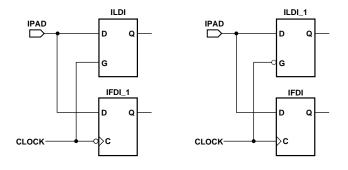
Figure 6-30 Legal Combinations of IFDI and ILDI for a Single IOB in XC4000E, XC4000X, Spartan, or SpartanXL
