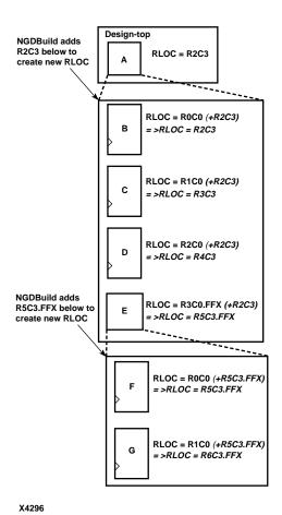
Figure 12-7 Adding RLOC Values Down the Hierarchy
