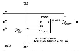
Figure 8-34 OFDT\_1 Implementation XC5200, Spartan2, Virtex
