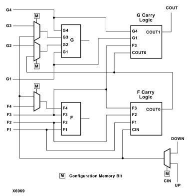
Figure 12-18 XC4000, Spartan, SpartanXL Carry Logic
