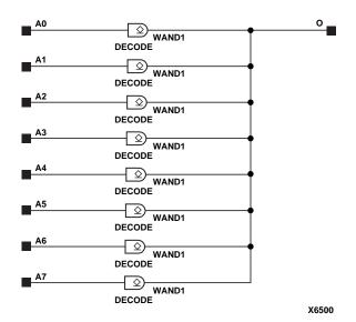
Figure 4-61 DECODE8 Implementation XC4000E, XC4000X
