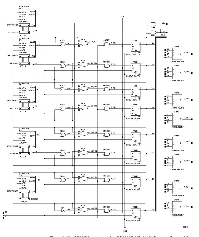
Figure 4-27 CC8RE Implementation XC4000E, XC4000X, Spartan, SpartanXL
