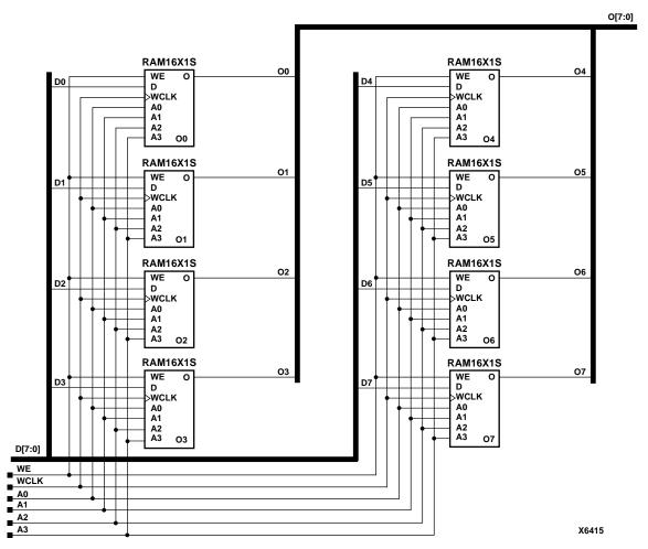
Figure 9-5 RAM16X8S Implementation XC4000E, XC4000X, Spartan, SpartanXL
