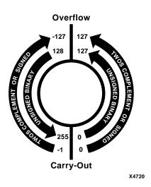
Figure 2-1 ADSU Carry-Out and Overflow Boundaries
