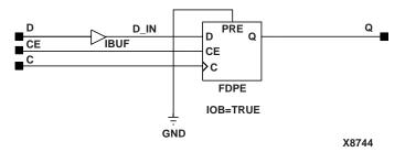
Figure 6-18 IFDXI Implementation Spartan2, Virtex
