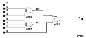
Figure 10-34 XOR8 Implementation XC4000E, XC4000X, XC5200, Spartan, SpartanXL
