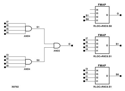
Figure 3-28 AND8 Implementation Spartan2, Virtex
