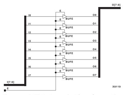
Figure 3-37 BUFE8 Implementation XC9000, Spartan2, Virtex
