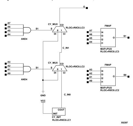
Figure 4-62 DECODE8 Implementation XC5200
