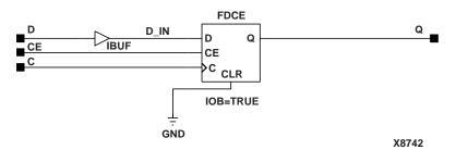
Figure 6-14 IFDX Implementation Spartan2, Virtex
