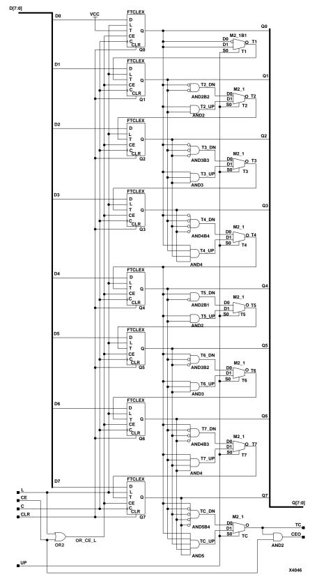
Figure 4-9 CB8CLED Implementation XC4000E, XC4000X, XC5200, Spartan, SpartanXL, Spartan2, Virtex
