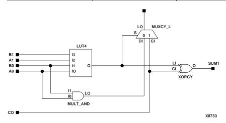
Figure 7-24 Example Multiplier Using MULT\_AND
