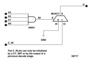
Figure 4-58 DEC\_CC4 Implementation Spartan2, Virtex
