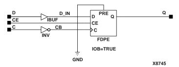
Figure 6-20 IFDXI\_1 Implementation Spartan2, Virtex
