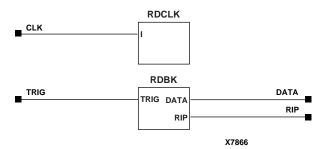
Figure 9-9 READBACK Implementation XC4000E, XC4000X, XC5200, Spartan, SpartanXL
