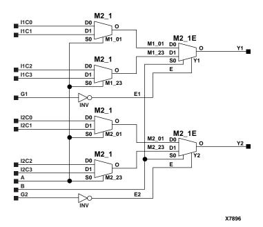
Figure 11-11 X74\_153 Implementation XC3000, XC4000E, XC4000X, XC5200, XC9000, Spartan, SpartanXL
