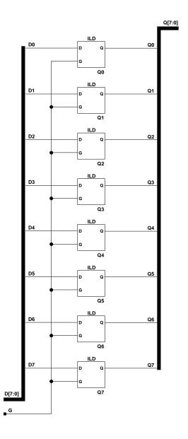
Figure 6-26 ILD8 Implementation XC3000, XC4000E, XC4000X, XC5200, XC9000, Spartan, SpartanXL, Spartan2, Virtex
