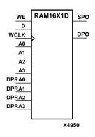
RAM16X1D is a 16-word by 1-bit static dual port random access memory with synchronous write capability. The device has two separate address ports: the read address (DPRA3 – DPRA0) and the write address (A3 – A0). These two address ports are completely asynchronous. The read address controls the location of the data driven out of the output pin (DPO), and the write address controls the destination of a valid write transaction.
