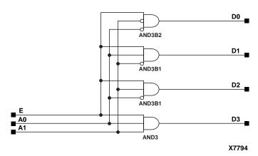
Figure 4-54 D2\_4E Implementation XC3000, XC4000E, XC4000X, XC5200, XC9000, Spartan, SpartanXL, Spartan2, Virtex
