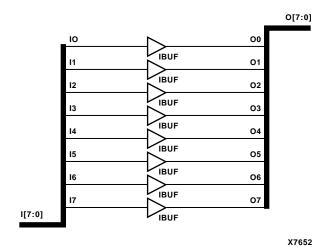
Figure 6-3 IBUF8 Implementation XC3000, XC4000E, XC4000X, XC5200, XC9000, Spartan, SpartanXL, Spartan2, Virtex
