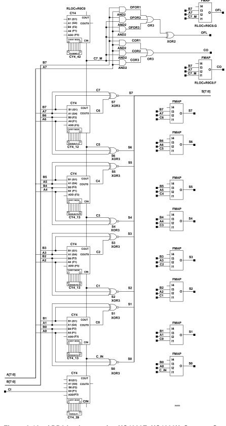
Figure 3-10 ADD8 Implementation XC4000E, XC4000X, Spartan, SpartanXL
