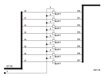
Figure 3-41 BUFT8 Implementation XC3000, XC4000E, XC4000X, XC5200, XC9000, Spartan, SpartanXL, Spartan2, Virtex
