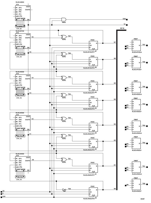
Figure 4-18 CC8CE Implementation XC4000E, XC4000X, Spartan, SpartanXL
