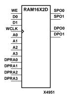
RAM16X2D is a 16-word by 2-bit static dual port random access memory with synchronous write capability. The device has two separate address ports: the read address (DPRA3 – DPRA0) and the write address (A3 – A0). These two address ports are completely asynchronous. The read address controls the location of data driven out of the output pin (DPO1 – DPO0), and the write address controls the destination of a valid write transaction.
