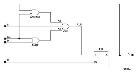
Figure 5-28 FDSE Implementation XC3000, XC4000E, XC4000X, XC5200, Spartan, SpartanXL
