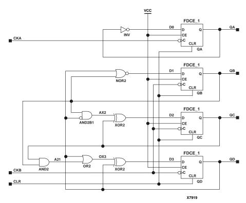
Figure 11-42 X74\_390 Implementation XC3000, XC4000E, XC4000X, XC5200, Spartan, SpartanXL
