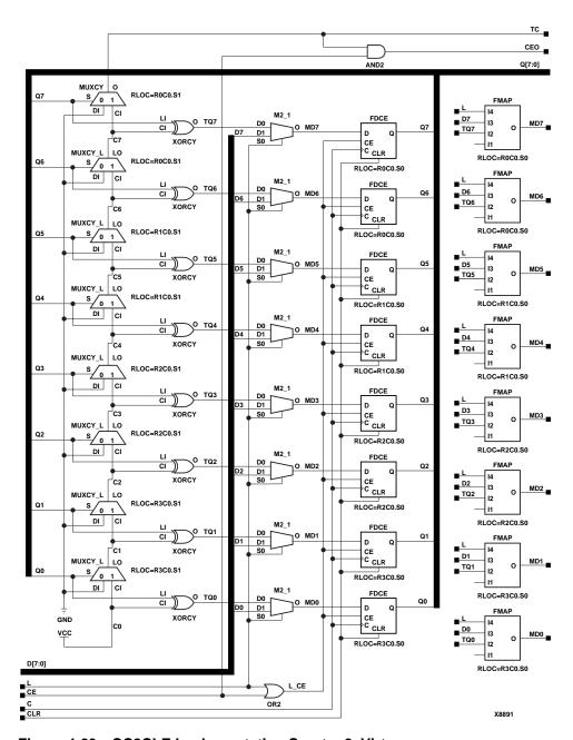
Figure 4-23 CC8CLE Implementation Spartan2, Virtex
