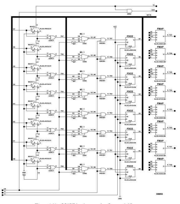
Figure 4-29 CC8RE Implementation Spartan2, Virtex
