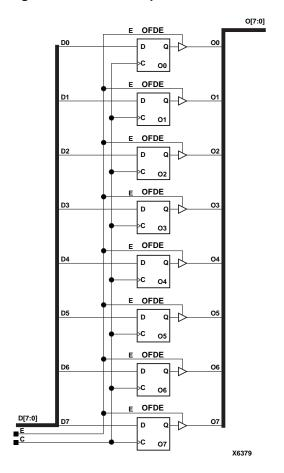
Figure 8-15 OFDE8 Implementation XC3000, XC4000E, XC4000X, XC5200, XC9000, Spartan, SpartanXL, Spartan2, Virtex
